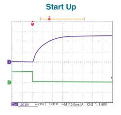
1. V<sub>OUT</sub> 20V/div 10mS/div 2. V<sub>OUT</sub> 5V/div 10mS/div
